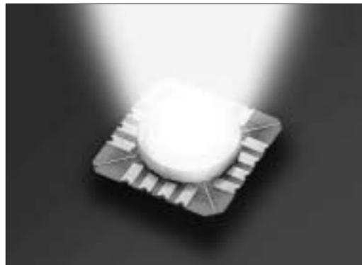
Citizen Electronics developed a commercial model of white power LED lamp for general lighting for the first time in autumn 2003. The new series features a luminous efficiency about 1.5 to 2 times higher than that of the original model, representing a significant advance in the luminous efficiency of LED lamps, which had been far lower than that of the fluorescent lamp.
